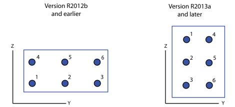
When constructing replicated subarrays using phased.ReplicatedSubarray, the GridSize and GridSpacing properties are used to position the subarrays on a rectangular grid. You specify the dimensions of the grid using the GridSize property and the distance between grid points with GridSpacing property. As with phased.URA, the interpretation of these properties has changed with this release. In this release, GridSize is a 1-by-2 vector in the form of [NumberOfRows NumberOfColumns] gives
